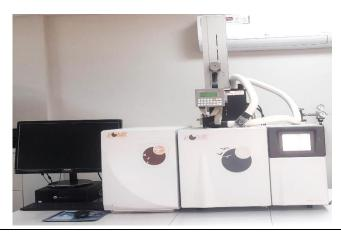
2. SHIMADZU Total Organic Carbon (TOC-L) Analyzer
