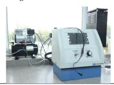
6. AQUASAFE WSL50 PRO Portable Field Laboratory (for the detection of microbiological and physico-chemical water quality parameters):
