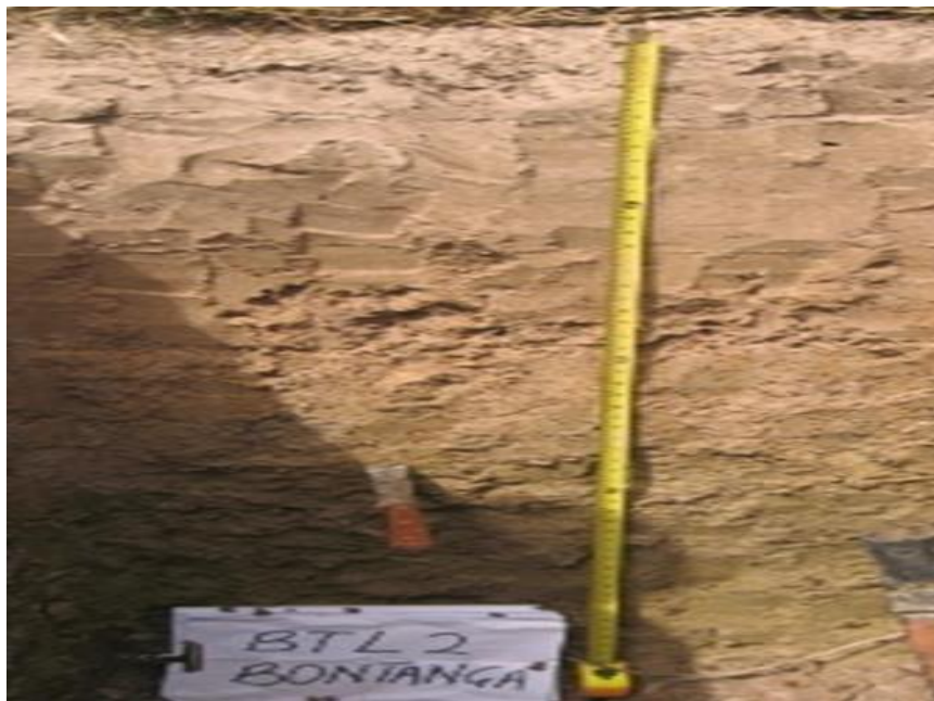
Figure 2.1: Typical Profile of Lima Soil Series (Source: Adapted from FAO/WRB: Endogleyi-Ferric Planosol in Buri et al. , 2012).
