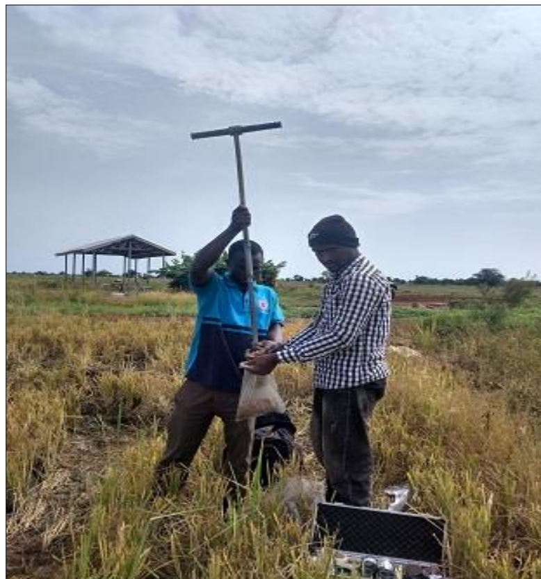
Plate 3.1: Field Soil Sampling using Auger
