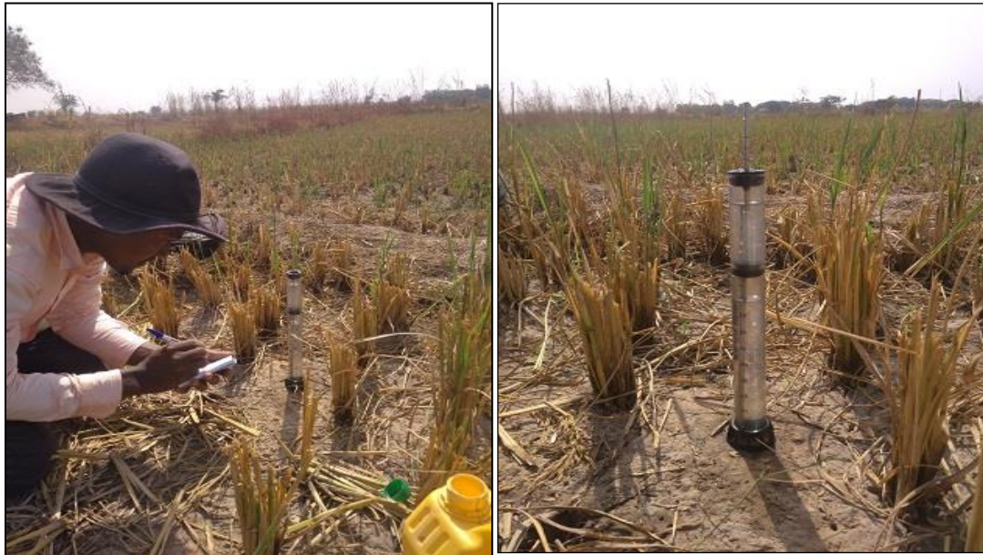
Plate 3.2: Conducting Infiltration Test Using Mini-disc Infiltrometer
